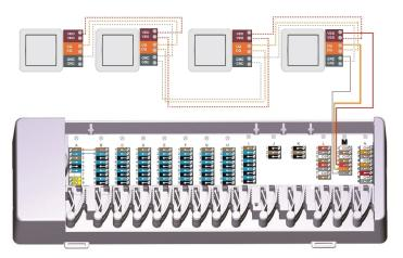
Example 2: Tree structure. Several stub lines lead from one main line to the individual sensors.
