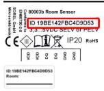
Each Room Sensor T2A has a unique 16-digit 1-Wire ID. This ID is required for sensor-room assignment in °CALEON. The ID can be found inside the sensor on the type plate and on the supplied sticker. We recommend placing the sticker in the table of the °CALEONbox instruction manual or in the °CALEONbox terminal plan sticker to simplify the later configuration of the system.
