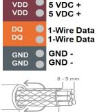
For the connection of a Room Sensor T2A, one of the terminal points VDD/ DQ/ GND is required in each case. The additional three clamping points are for easy connection of further sensors. Use a suitable twisted pair cable and ensure sufficient wire cross-section e.g. LIYCY 2 x 2 x 0.75mm<sup>2</sup>
