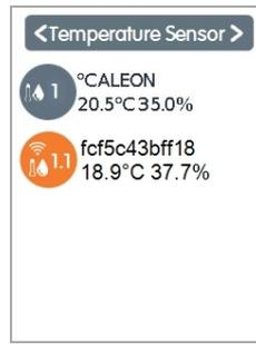
Select the Room Sensor Smart as the temperature sensor. The sensor can be identified by the MAC address shown on the display/ type plate.
