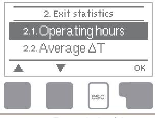
The menu "2. Statistics" is used for function control and long-term monitoring of the system.
