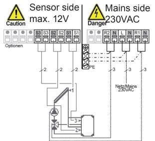
Actuating direction of valve: R2 on/valve on = charge to sensor 3 (storage tank above)
