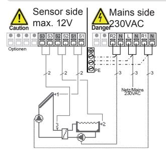
Relay R1: For speed control of standard pumps, minimum load 20VA
