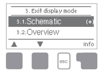
Menu "3. Display mode" is used to define the controller's display for normal operation.
