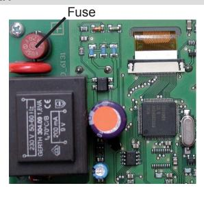
If the mains voltage is switched on and the controller still does not function or display anything, then the internal device fuse may be defective. In that case, open the device as described under C, remove the old fuse and check it. Exchange the defective fuse for a new one, locate the external source of the error (e.g. pump) and exchange it. Then first recommission the controller and check the function of the switch outputs in manual mode as described under 4.2.
