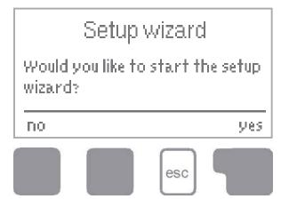
The first time the controller is turned on and after the language and time are set, a query appears as to whether you want to parametrise the controller using the commissioning help or not. The commissioning help can also be terminated or called up again at any time in the special functions menu. The commissioning help guides you through the necessary basic settings in the correct order, and provides
