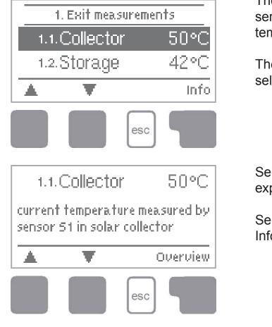
The menu "1. Measurement values" serves to display the currently measured temperatures.
