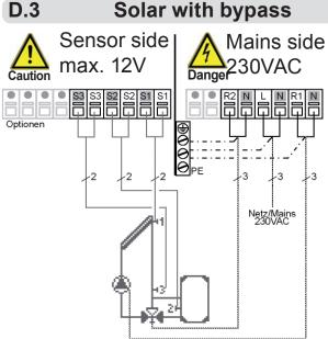
Actuating direction of valve: R2 on/valve on = bypass without storage tank charging
