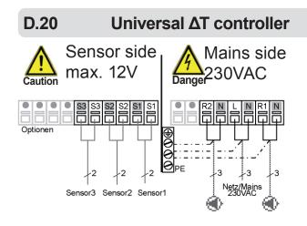
Brief description of switching function: The  $\Delta T$  function sensor 1 > sensor 2 switches the pump to relay R1. The thermostat function via sensor 3 switches the pump to relay R2.
