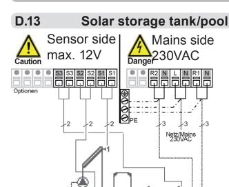
Actuating direction of valve: R2 on/valve on = charge to sensor 3 (swimming pool)
