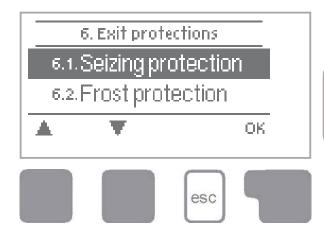
Menu "6. Protective functions" can be used to activate and set various protective functions.
