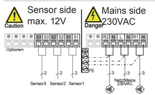
Brief description of switching function: The  $\Delta$ T function sensor 1 > sensor 2 switches the pump to relay R1. The  $\Delta$ T function 2 > sensor 3 switches the pump to relay R2.
