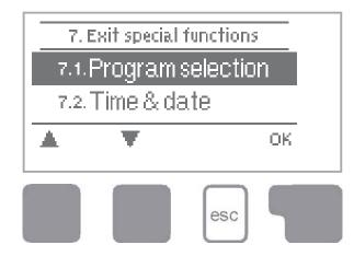
Menu "7. Special functions" is used to set basic items and expanded functions.
