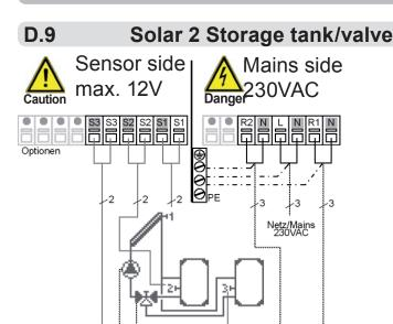
Actuating direction of valve: R2 on/valve on = charge to sensor 3 (storage tank 2)
