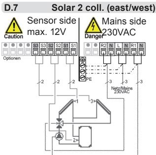
Actuating direction of valve: R2 on/valve on = collector with flow through
