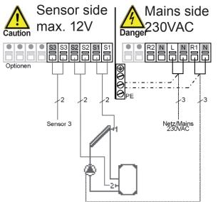
Relay R1 and R2 are both switched on in this variant, so e.g. a pump can be connected to R2.
